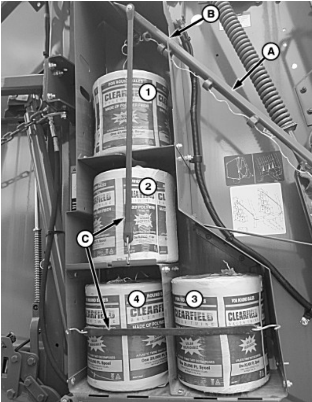
A—Twine Guide Arm B—Twine Box Notch C—Strap (2 used)
