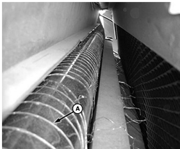
Net Material Against Steel Roll
