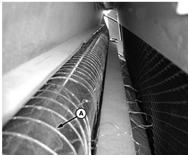
Photo 1—Timing is Correct (Net Wrap Material is Snug Against Steel Roll)
