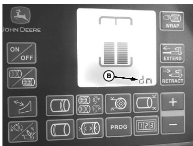
A—“up”—Raised Position B—“dn”—Lowered Position
