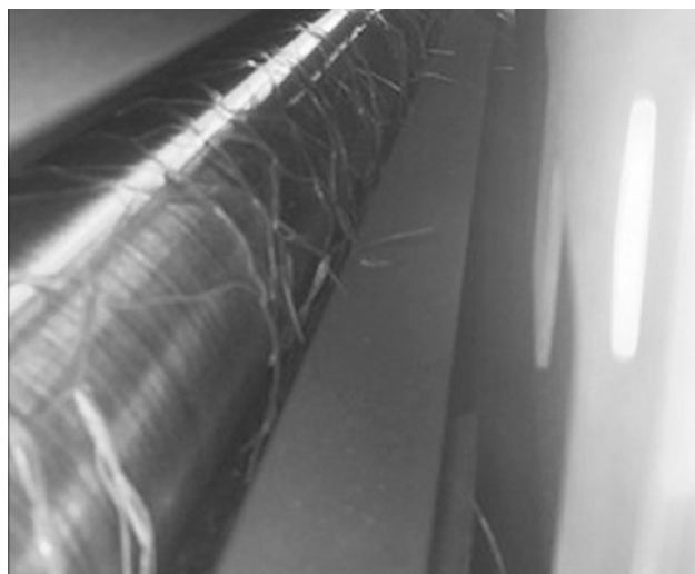
Photo 3—Timing is Early (Broken Net Material Has Snapped Back)
